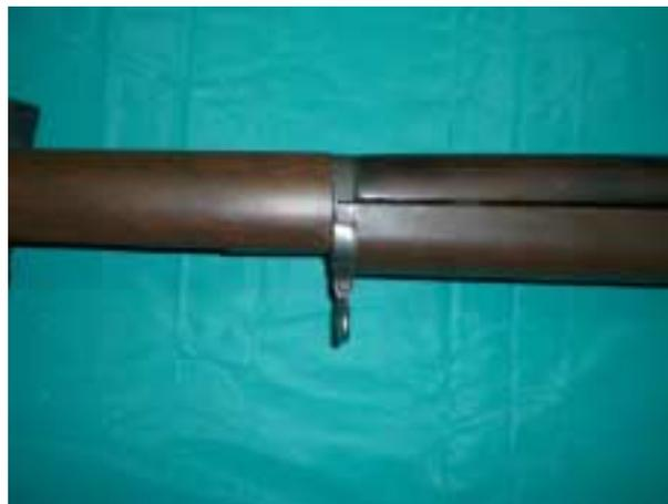
18. The final part of the assembly is to re-connect the stock. Follow the disassembly steps in reverse order. Once the stock is in place you will need to take a strip of black electrical tape, cut it in half (length wise) and wrap it around the front of the stock and the Rear
