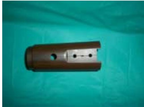
11. You will now need to trim the inside of the stock, at the new cut, so that it will fit around the Lower Band of the Handguard. I used the Dremel for this part and worked slowly checking the fit and making any additional trimming as needed. The plastic almost melts as you are making these small cuts so be very careful.
