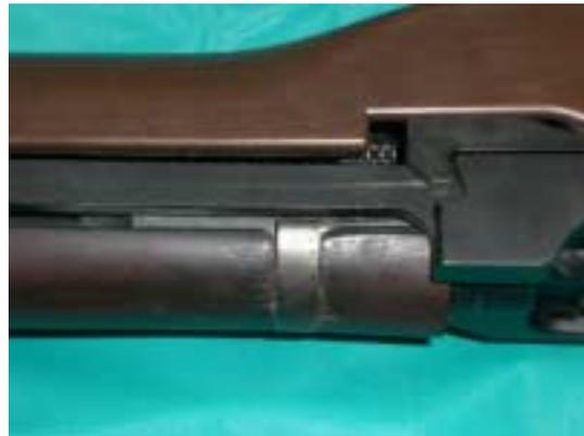
9. Now that you have cut down the rear hand guard you will also need to adjust the section of the rear hand guard that meets the stock so that the bolt slide will fit. I used the Dremel to make the cuts. Take your time with these cuts. Cut across 5/8 and then cut at an angle the same length. Better to make small cuts and check the fit.
