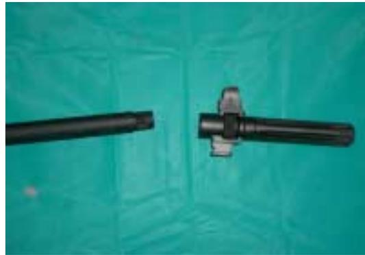
4. Next, remove the Gas Cylinder assembly by using the 1.5 Allen key to unscrew the Gas Cylinder assembly screw. Once the assembly is free remove it from the barrel.
