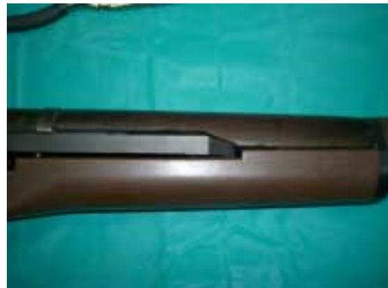
10. Mark off 3 ¾ inches from the front end of the plastic stock. This should be just at the one end of the swing swivel. Note: I used black electrical tape to mark off the cut off line. Make the cut.
