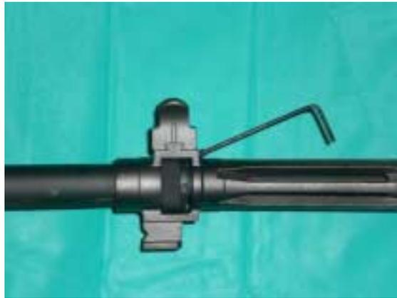
3. Once the Flash suppressor set screw is far enough back (you do not need to remove it) you can then unscrew the Flash suppressor nut off and remove the Flash suppressor from the barrel.
